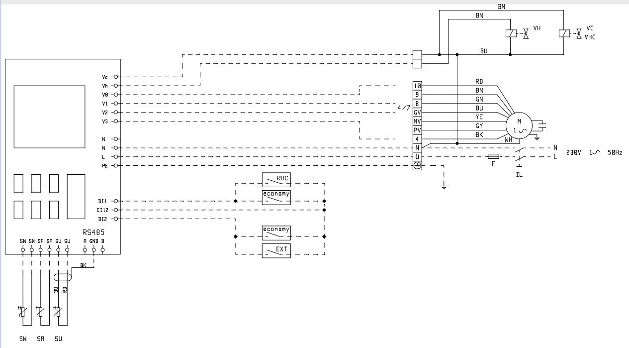
» Electrical connection FWEC2A/3A + FWB-C 15-17 + valve - Collegamento elettrico FWEC2A/3A + FWB-C 15-17 + valvola - Branchement électrique FWEC2A/3A + FWB-C 15-17 + vanne - Elektrischer Anschluss FWEC2A/3A + FWB-C 15-17 + ventil - Conexión eléctrica FWEC2A/3A + FWB-C 15-17 + valvula
