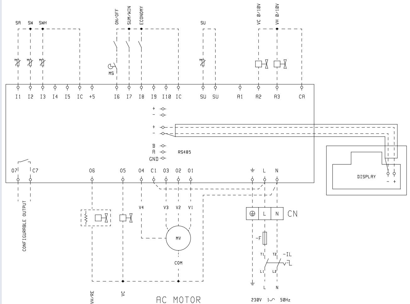
» Electrical connection FWEC1A + FWB-C 04 + valve - Collegamento elettrico FWEC1A + FWB-C 04 + valvola - Branchement électrique FWEC1A + FWB-C 04 + vanne - Elektrischer Anschluss FWEC1A + FWB-C 04 + ventil - Conexión eléctrica FWEC1A + FWB-C 04 + valvula
