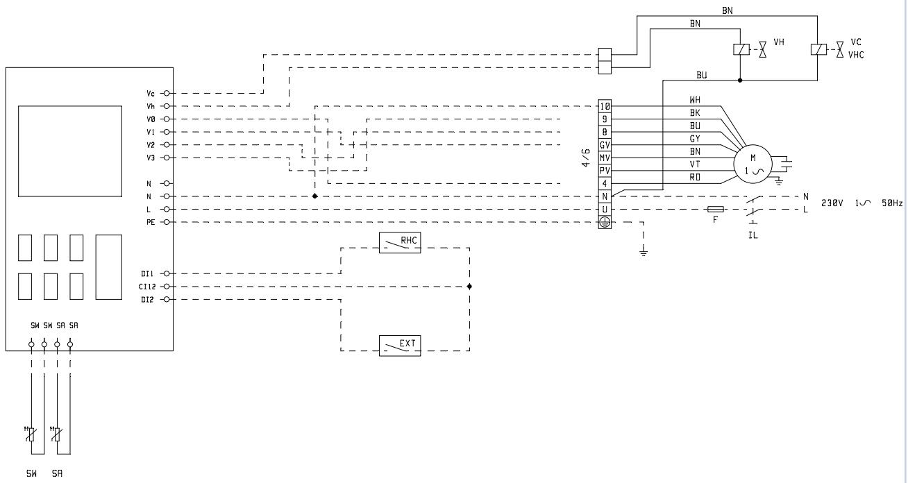
» Electrical connection FWEC1A + FWB-C 05-11 + valve - Collegamento elettrico FWEC1A + FWB-C 05-11 + valvola - Branchement électrique FWEC1A + FWB-C 05-11 + vanne - Elektrischer Anschluss FWEC1A + FWB-C 05-11 + ventil - Conexión eléctrica FWEC1A + FWB-C 05-11 + valvula
