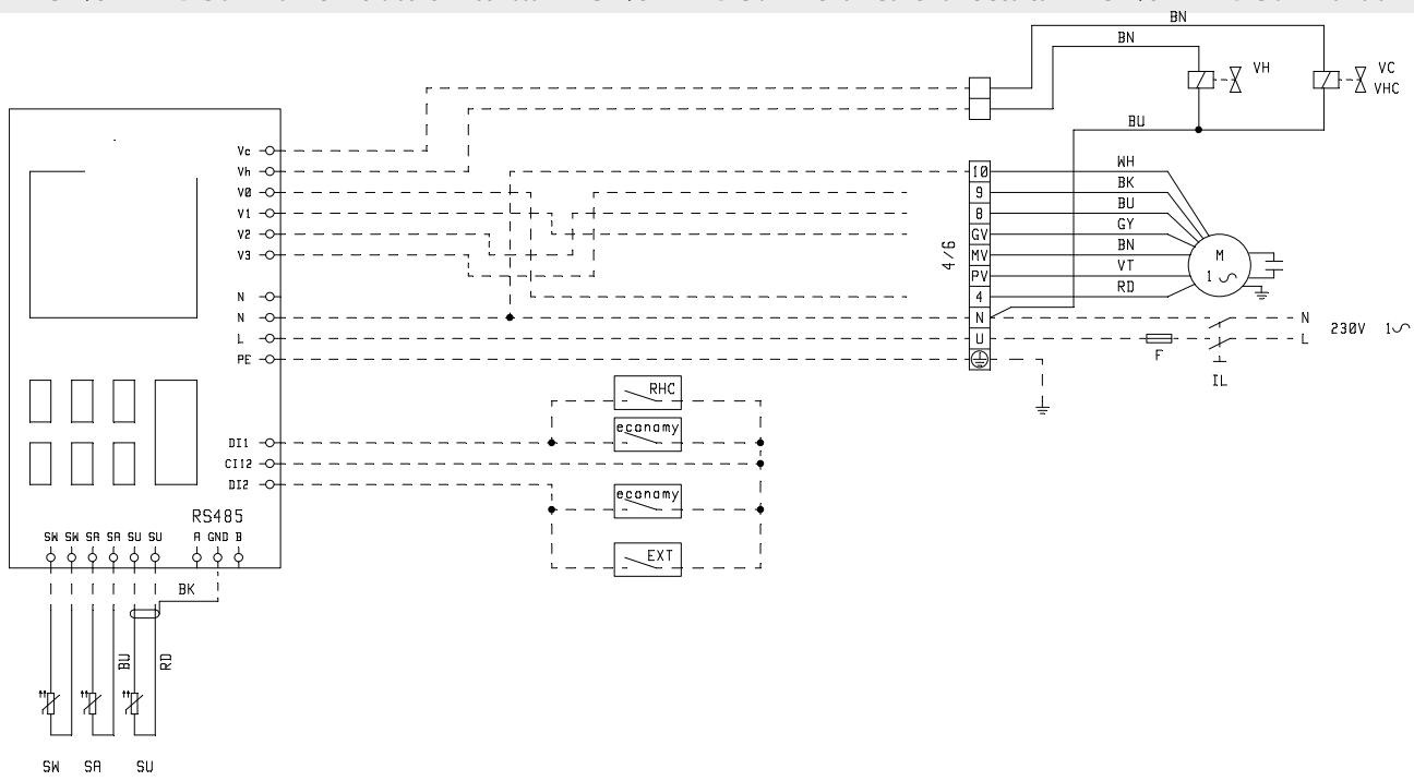
» Electrical connection FWEC2A/3A + FWB-C 5-11 + valve - Collegamento elettrico FWEC2A/3A + FWB-C 5-11+ valvola - Branchement électrique FWEC2A/3A + FWB-C 5-11 + vanne - Elektrischer Anschluss FWEC2A/3A + FWB-C 5-11 + ventil - Conexión eléctrica FWEC2A/3A + FWB-C 5-11 + valvula
