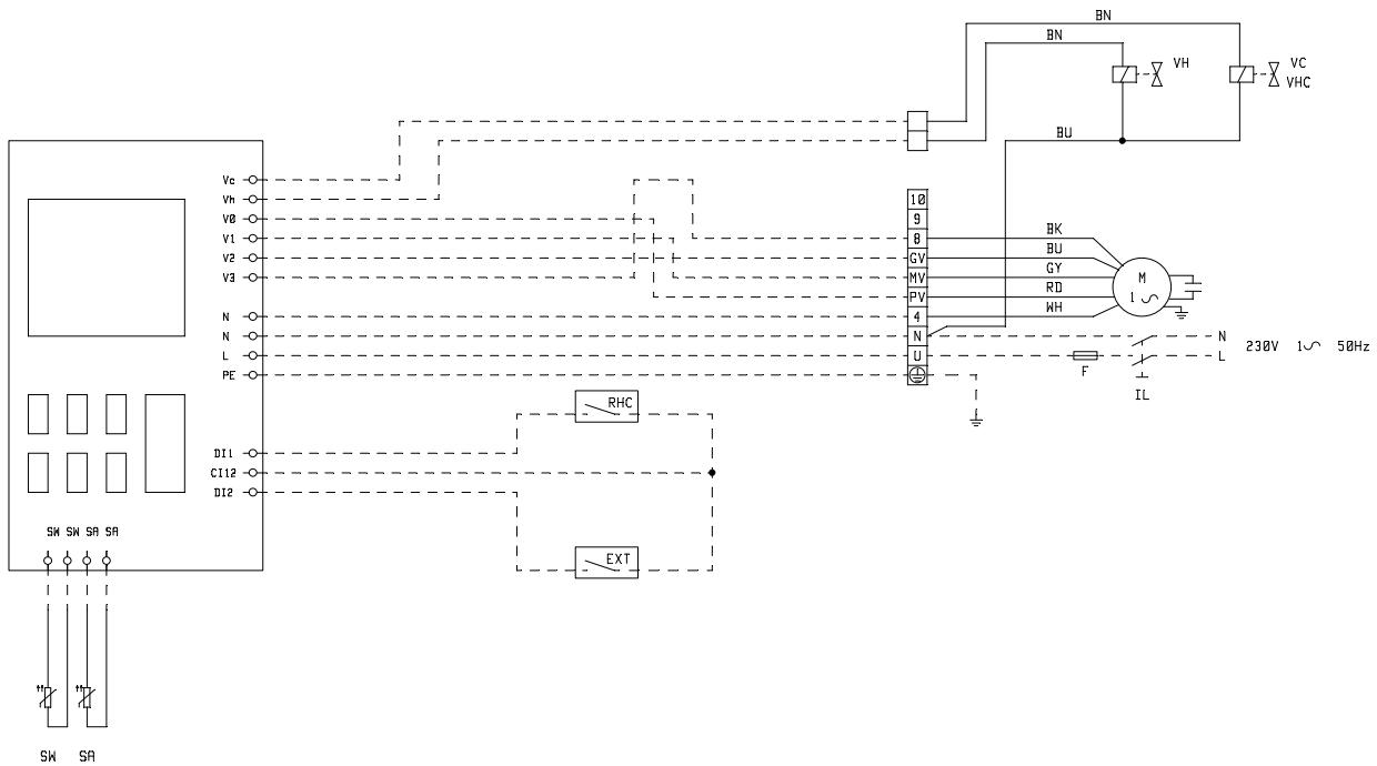
» Electrical connection FWEC2A/3A + FWB-C 04 + valve - Collegamento elettrico FWEC2A/3A + FWB-C 04 + valvola - Branchement électrique FWEC2A/3A + FWB-C 04 + vanne - Elektrischer Anschluss FWEC2A/3A+ FWB-C 04 + ventil - Conexión eléctrica FWEC2A/3A + FWB-C 04 + valvula
