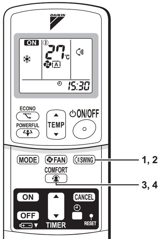
The diagram shows a DAIKIN remote control. The LCD screen displays 'ON', a temperature of 27°C, a fan icon, and a time of 15:30. Below the screen are buttons for 'ECONO', 'POWERFUL', 'TEMP', and 'ON/OFF'. The lower section of the remote features 'MODE', 'FAN', 'SWING', and 'COMFORT' buttons. At the bottom are 'ON', 'OFF', 'TIMER', 'CANCEL', and 'RESET' buttons. Lines with numbers 1, 2, 3, and 4 point to the SWING, FAN, and MODE buttons respectively.
