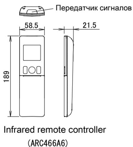
Infrared remote controller (ARC466A6)
